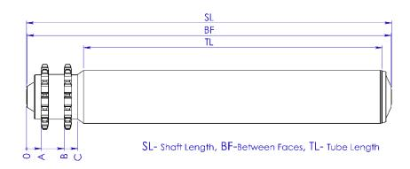
The AIROLL Series 100 Chain Driven Conveyor Rollers are ideally suited to be fitted in light duty and medium duty roller conveyors. conveying containers, pallets, drums as well as other light and medium unit loads.
