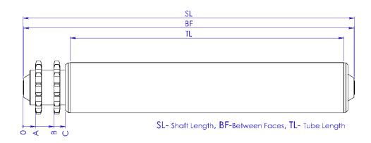
The Airoll Series 200 Chain Driven Conveyor Rollers are especially suited to convey heavy duty materials like pallets, containers, drums and other heavy unit loads.
