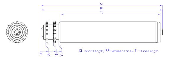
The AIROLL Series 300 medium duty Chain Driven Conveyor Roller is a stronger option than the Series 100. It is remarkably robust and is the most popular and economically priced of all our conveyor rollers. The Series 300 conveyor roller is specified and fitted in most newly built gravity roller conveyors.
